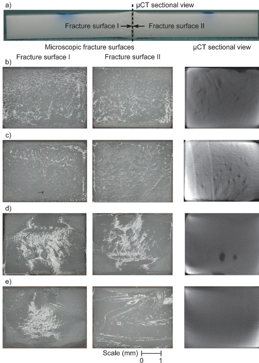
Figure 3: a) Microscopic overview of fracture surfaces I and II ( $200\times$ ) and position of the  $\mu$ CT sectional view ( $9.2\ \mu\text{m}$  resolution) of, b) specimen in group Ia-GS2 with minimum bending strength of 52.8 MPa, c) specimen of group Ia-GS2 with maximum bending strength of 83.9 MPa, d) specimen of group IIa-GS2 with minimum bending strength of 89.1 MPa, d) specimen of group IIa-GS2 with maximum bending strength of 217.0 MPa
